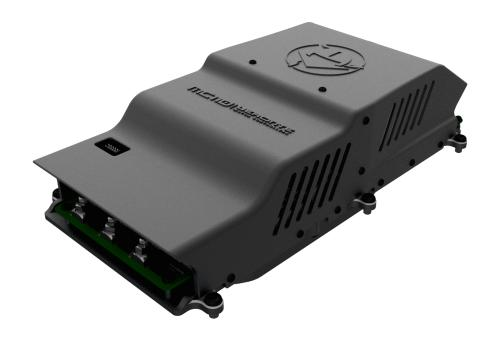
**Veronte MC110** speed controller is capable of driving any type of 3-phase PMSM motor. It can be used with a wide variety of UAVs or eVTOL vehicles. **MC110** uses FOC algorithm for motor control together with IGBTs.
